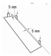
1. Start with a first, full length plank (n°1), which comes in the top left corner of your room. Preferably lay the 2 sides with tongue towards the walls and make sure that the expansion joint of 5 mm is respected. The groove or tongue is not part of the expansion joint. Cut them off if necessary.
